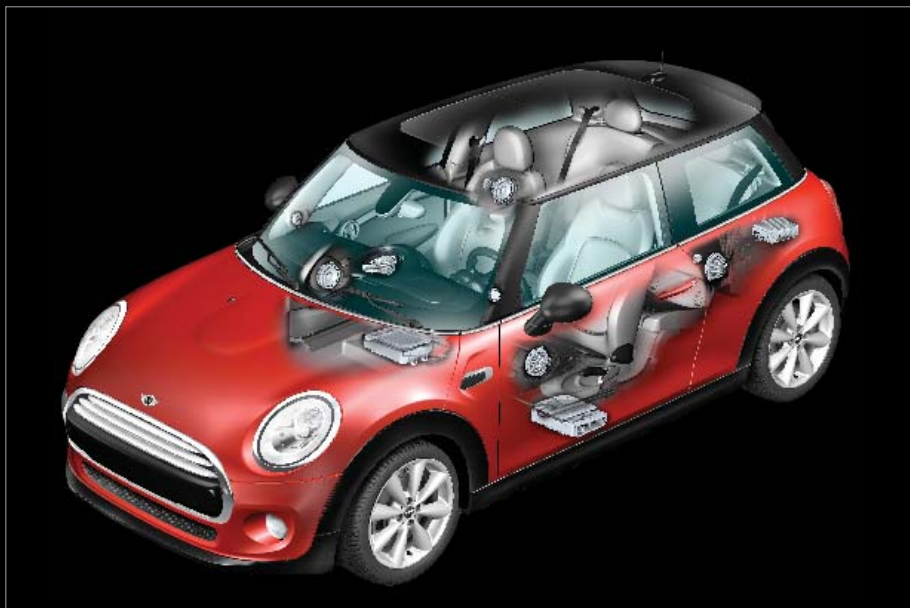
674- Hi-fi loudspeaker system harman/kardon (12 speaker system with DSP amplifier) layout
