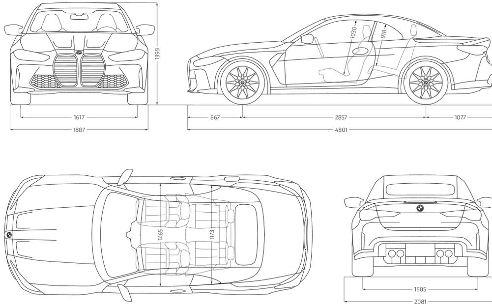
The dimensions in the technical drawing are in millimetres and may vary depending on the model and the optional equipment.
