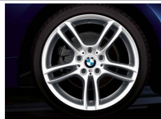
M Double Spoke - Style 261M 7.5J x 18 front / 8.5J x 18 rear 215/40 R 18 front / 245/35 R 18 rear Performance Run-Flat Tires*
