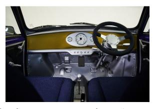
Smith's design leaves out entire instruments in other places: a magnet next to the steering wheel accommodates the smartphone, which, apart from the speedometer, replaces almost all the old buttons and functions on the dashboard. The steering wheel in his exclusive model can be completely removed to facilitate getting in and out of the car – both an innovative solution as well as a tongue-in-cheek quip symbolic of Paul Smith's trademark wit.
